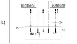
Step.3: Secure lamp body to outlet box, and use additional anchors when needed.
