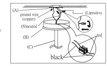
Step.3: Wire fixture to wires in outlet box. Install green wire to ground screw.
