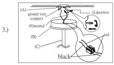
Step.3: Wire fixture to wires in outlet box. Install green wire to ground screw.
