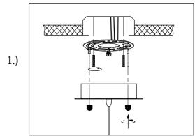
Step.1: Remove mounting bracket (A) from fixture and install to electrical box.
