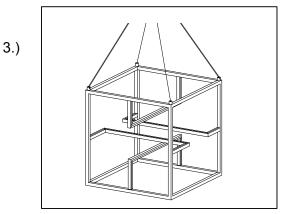
Step.3: Adjust wire length to desired mounting height, and tighten strain relief screws to secure.
