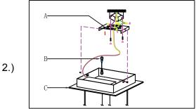
Step. 2: Connect safety lanyard(B) to Mounting Bracket(A). Wire fixture to wires in outlet box. Bare wire is for Ground. Secure canopy(C) to mounting bracket using screws on the sides of the canopy.
