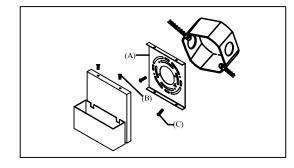
Step 1: Remove mounting bracket from fixture and install to electrical box.
