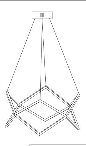
WARNING: Wires need to be connected to driver found in canopy and should not be connected directly to power source or a short may occur.
