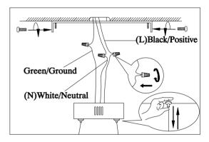
Step 2:Adjust wire length to desired mounting height, and tighten strain relief screws to secure. Wire fixture to wires in outlet box. Green wire is for ground.
