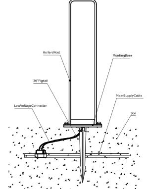
NOTE: Alumilux pathway light is provided with a ground stake to facilitate an in-grade installation. However, for a permanent and secure installation a concrete footing support for bollard post is recommended.
