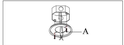
Step.1: Install Backplate(A) to outlet box.
