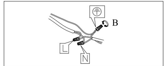
Step.2: Wire fixture to wires in outlet box. Green/Copper wire is for Ground.
