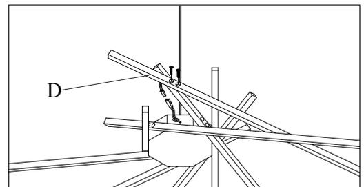
Step.4: Using the quick connect plug, wire the LED arm (D) to the fixture body. Secure to the body of the fixture using screws provided.
