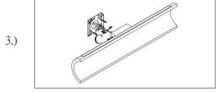
Step.3: Caulk around fixture with outdoor silicone sealant to prevent water intrusion. Leave a small gap at the bottom to allow moisture to escape. Install fixture to mounting bracket(A) and tighten mounting screws (C) to secure.
